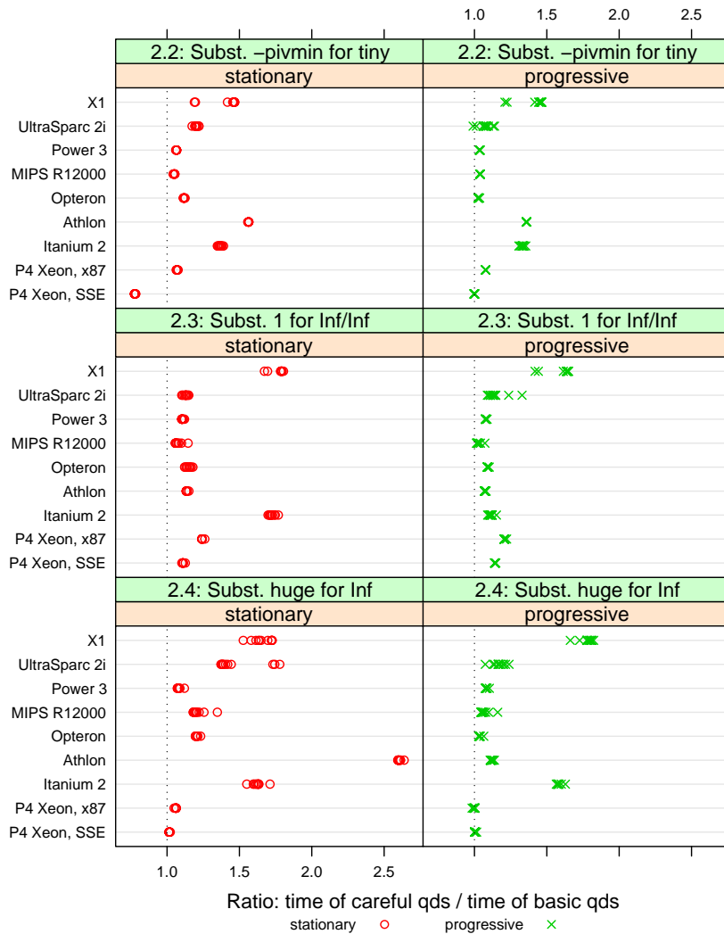
Fig. 3.4: As long as no exception occurs, the basic qds loop almost always runs faster than the careful loops that test for exceptional operations. A point at 1.2 means the careful loop’s running time was 1.2 times the basic loop’s time; the basic loop sees a speed-up of 20%.
