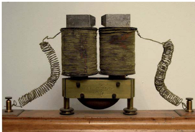
Fig. 6. Electromagnet used by Bancalari in his research on the magnetic properties of gases, apparently taken from a Pixii machine.
