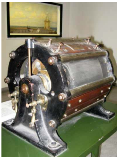
Fig. 15. Gramme AC ring-armature generator with 4 circuits to feed four Jablochkoff arc lamps, 1878 (inv.-no.12682)
