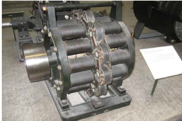
Fig. 10. Hefner-Altenneck AC generator with disc armature, 1878 (inv.-no. 33611)
