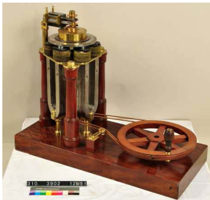
Fig. 3. Stöhrer's machine with disc armature, 1863 (inv.-no. 3902)
