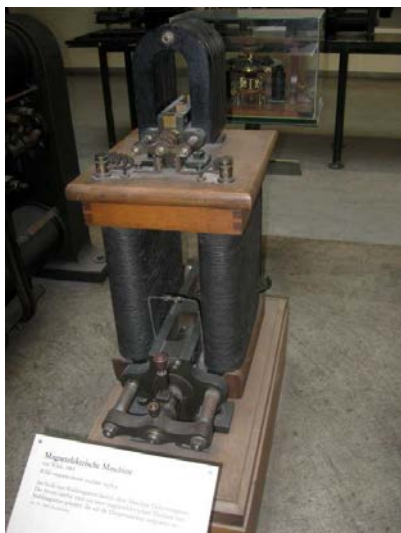
Fig. 7. Wilde's magneto-electric machine with external excitation, 1865 (inv.-no. 72434, replica)
