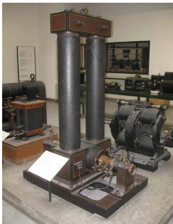
Fig. 35. Z-type "Long-Legged Mary Ann", Edison's first commercial dynamo, 1879 (inv.-no. 18326)
