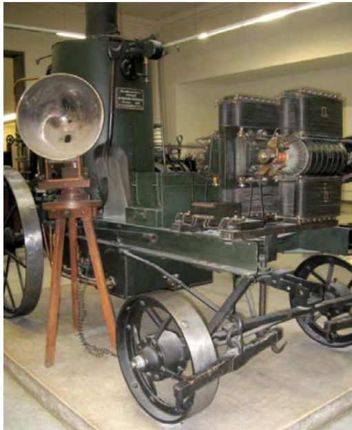
Fig. 33. At left: a double-dynamo in a horse-drawn vehicle (movable furnace and boiler) for arc light, 1878 (inv.-no. 20205). At right detail, seen from reverse side (inv.-no. 20205)
