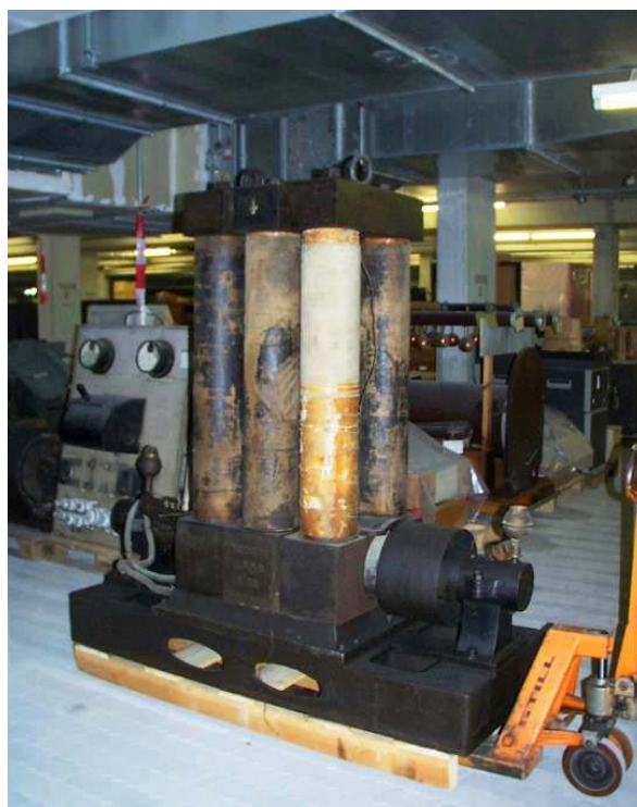
Fig. 36. Edison's K-type dynamo, 1882 (inv.-no. 17395)
