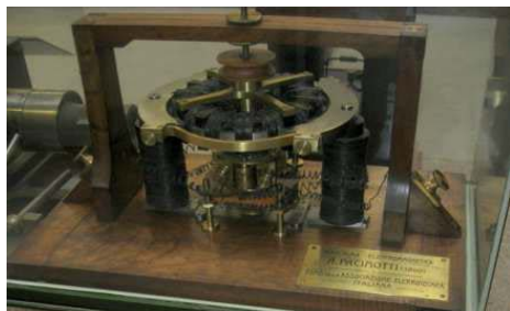
Fig. 22. Pacinotti's ring armature generator, 1860 (replica, inv.-no. 7862)
